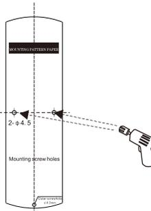
2. Attach the installation paper to the wall, mark the holes first and then make the guide holes.
