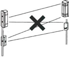
4. Avoid any other detector interference (stack installation only for same model)
