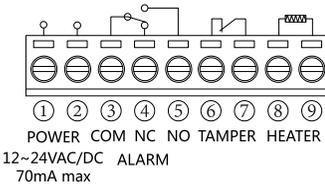
1. Power voltage input: DC/AC12V-24V.
