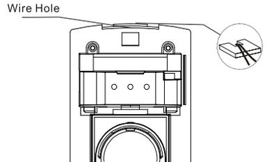
3. Drop into the holes with expansion pipe, leave a 10cm-long wire for connection, then fix it with screws.
