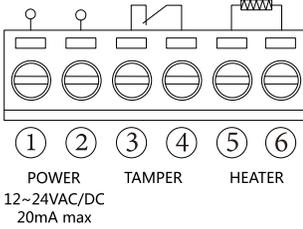
1. Power voltage input: DC/AC12-24V
