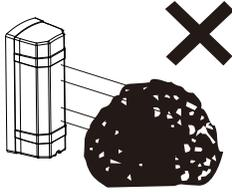
2. Do not install the unit where objects can block the beams like the plants and laundry can be moved by wind
