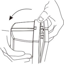
1. Loosen the screw and remove the cover
