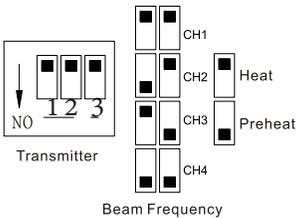
1. DIP switch 1 & 2 position should be the same on transmitter and receiver (Two or more pairs beams installed on the same plane, recommend user set to different frequencies for each adjacent pair to avoid mutual interference between beams).
