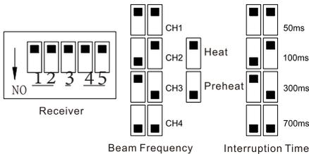
1. DIP switch 1 & 2 position should be the same on transmitter and receiver (Two or more pairs beams installed on the same plane, recommend user set to different frequencies for each adjacent pair to avoid mutual interference between beams).
