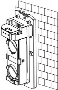
4. Drop into the two holes with the expansion pipes, fix them with screws.
