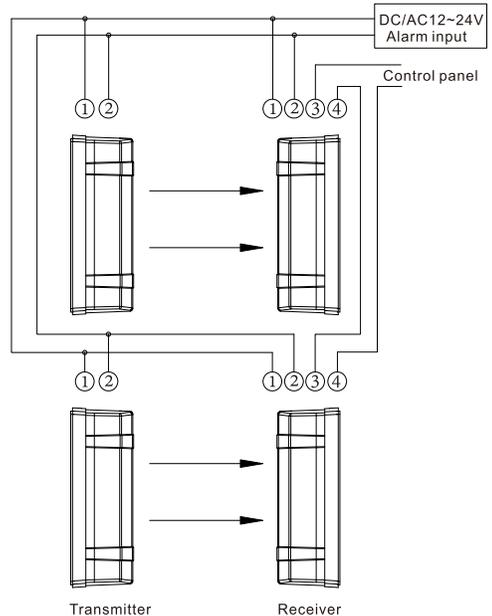
(3).2 pairs install in series: Connect power of transmitter and receiver in series with 12V DC on power supply. Alarm output is N.C.
