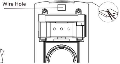
3. Wiring hole: Remove the foam plug, pull wire through, leave a 10cm-long wire for connection and reset the foam plug.
