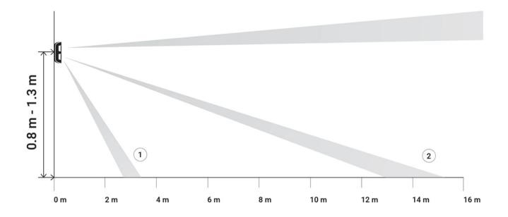
The detection distance is adjusted using the **Detection Distance** scrollbar on the rear panel of the detector. When choosing the installation location, consider the maximum detection range of the detector. It depends on the sensitivity, the position of the Detection Distance scrollbar, the type and speed of the person's movement (running, walking), and the ambient temperature.
