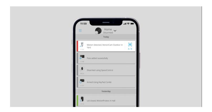
If the **Send photo in case of alarm** option is enabled for MotionCam Outdoor, alarms in Ajax apps will be accompanied by a series of photos (the number depends on the settings). To view the photos, click on the alarm notification in the events feed.
