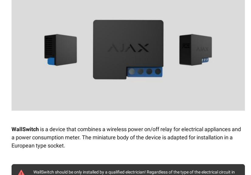
WallSwitch operates only with the Ajax security system (it may not be used in any third-party security systems), by connecting via the protected Jeweller protocol to the hub. Communication range – up to 1,000 meters, absent any obstacles. Use scenarios to program actions of automation devices (Relay, WallSwitch or Socket) in response
