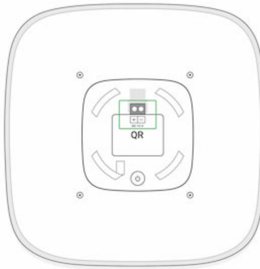
6. Place the front side of the siren on a hard surface and unscrew the 4 screws on the rear panel with a PH2 screwdriver.
