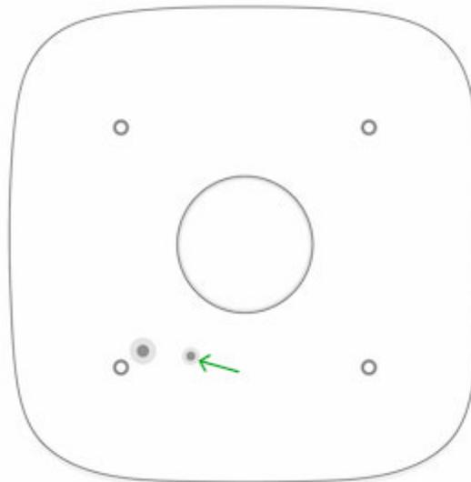
**11.** Fit the protective plastic panel in place (the Ajax logo on the connection side of the LED strip to the board) with little effort. The properly mounted plastic panel will protrude above the
