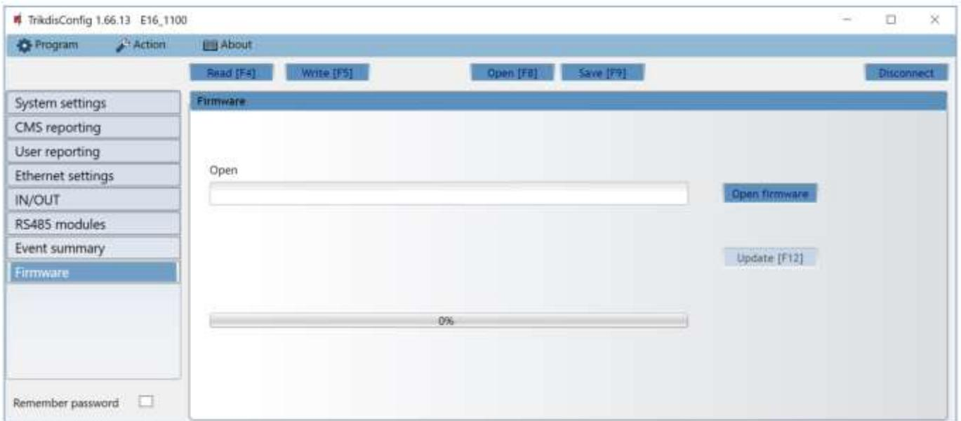
4. Press **Open firmware** and select the required firmware file. If you do not have the file, the newest firmware file can be downloaded by registered users from [www.trikdis.com](http://www.trikdis.com), under the download section of the **E16** communicator.
