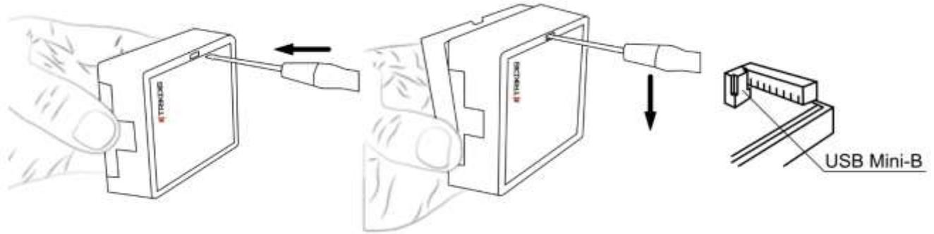
3. Using a USB Mini-B cable connect the *E16* to the computer.
