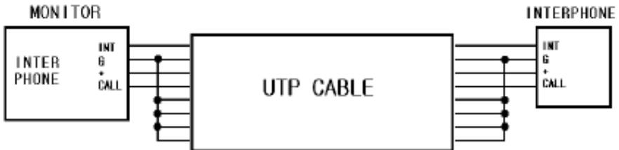
If you use UTP CABLE[CAT.5], connect the rest 4 lines to GND after connecting 4 lines between monitor and interphone.
