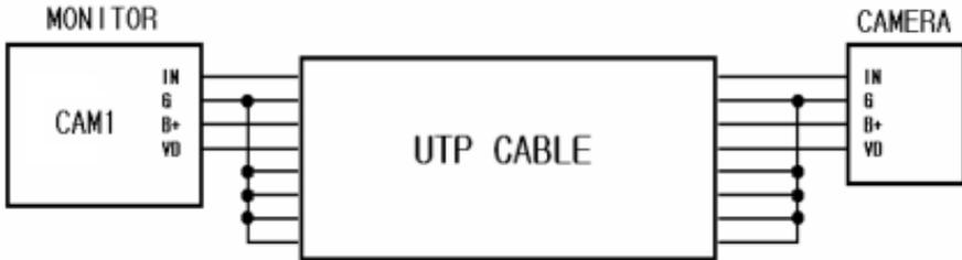
If you use UTP CABLE[CAT.5], Connect the rest 4 lines to GND after connecting 4 lines between monitor and camera.
